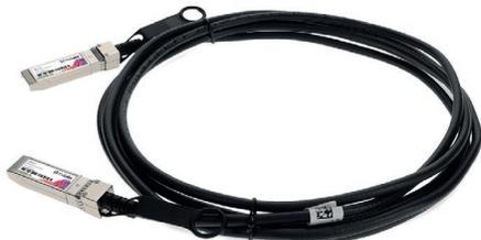
Passive copper Direct Attach Cables (DAC) are a low cost alternative for short reach applications. The passive design has no signal amplification in the cable assembly. Electronic dispersion compensation (EDC) is typically used on host board designs when passive copper cable assemblies are utilized. They are ideal for short distances up to 10 meters and offer a cost effective solution for connecting compatible OEM equipment within a rack.
